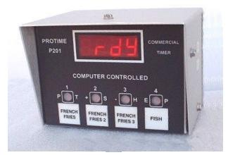
The **PROTIME 2** is a four product timer that has been designed to provide quality at a low cost. Programming all parameters: cooking times, stir times, and hold times is easily done from the front panel. There are two stir times per channel. Timing accuracy is maintained by use of a precision ceramic resonator.
